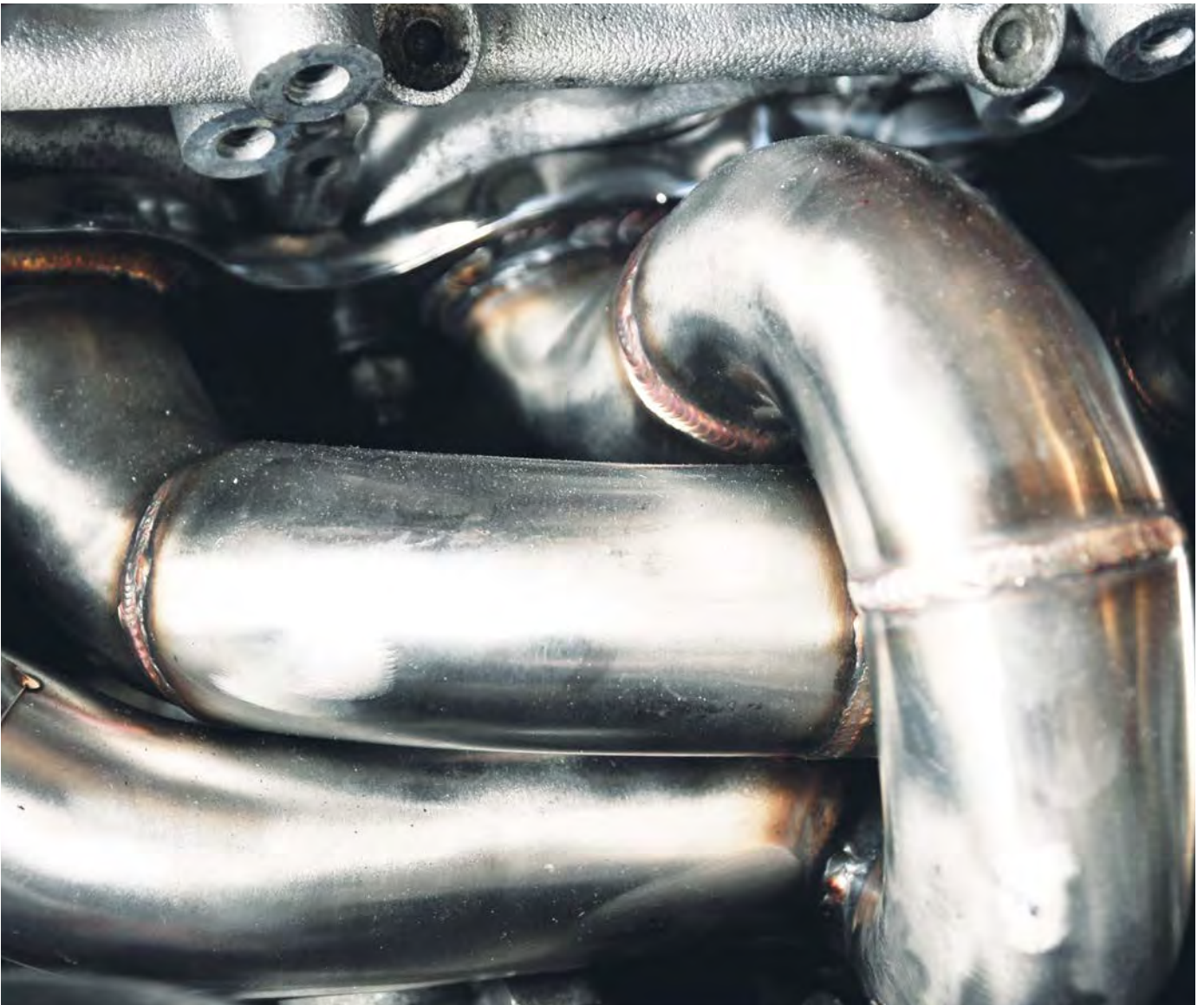
Weld seams on an exhaust manifold
